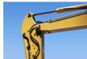
Hydraulic hoses for construction equipment
