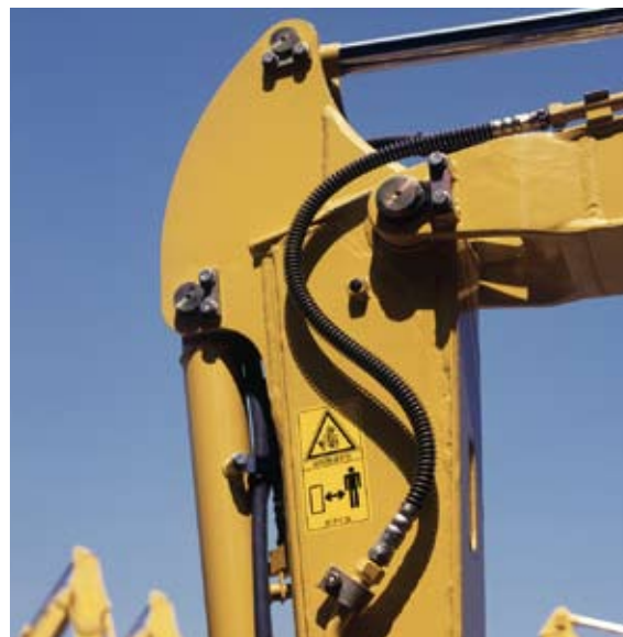
Yokohama high-pressure hoses convey hydraulic power for this power shovel.
