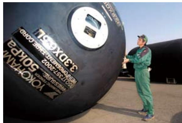
This Yokohama marine fender is 3.3 meters in diameter and fully 6.5 meters long.
