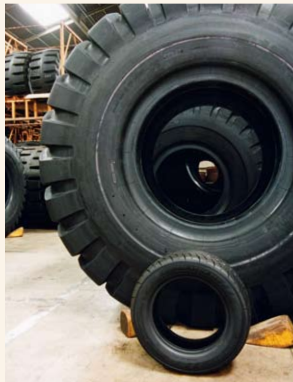
The big off-the-road tire in the photo has an inner diameter of 35 inches. A passenger-car tire puts the matter of size in perspective.
