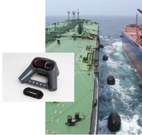
High-performance fenders. Yokohama's Fender Watch system for pneumatic marine fenders allows for remote monitoring of the air pressure in the fenders with the sensor and monitor shown here. That simplifies maintenance work greatly at offshore oil rigs and at other marine settings.
