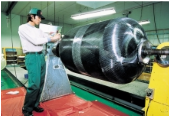
Our water tanks for airplane use are strong, yet light, thanks to the wrapping of a multilayer compound of epoxy resin and carbon fibers.
