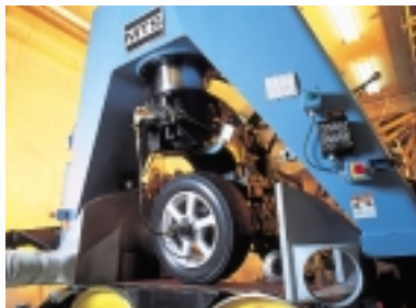
Testing machine for studying tire characteristics during cornering.
