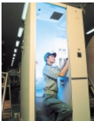
Yokohama's lavatory modules for Boeing are made with our Advanced Composite Material to achieve high strength at a low weight.
